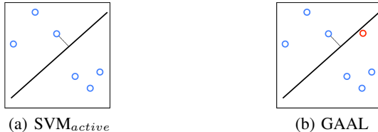
Figure 3: (a) SVM_{\text{active}} algorithm selects the instances that are closest to the boundary to query the oracle. (b) GAAL algorithm synthesizes instances that are informative to the current learner. Synthesized instances may be more informative to the learner than other instances in the existing pool.
